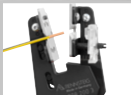
Automatic stripping of the insulation.
