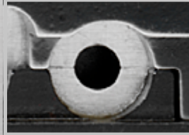
Stripping Area (Round Blades, no wire damage)
